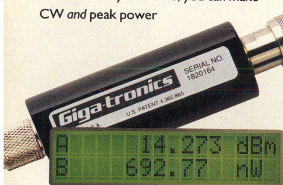
The two-line display also lets you set the desired resolution and select either Lin or Log readout for each line.
